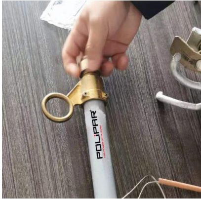
3. Loosen the cap of the fuse tube
